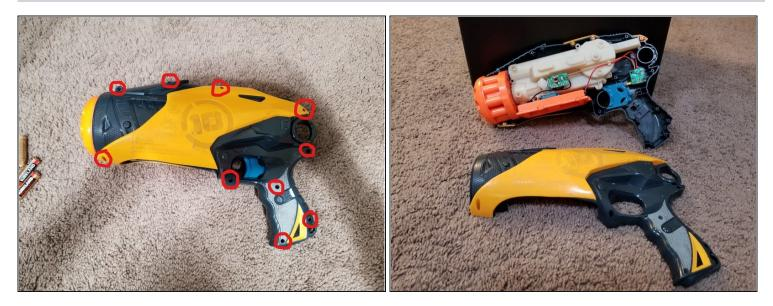
• After removing the batteries you want to use the screwdriver to unscrew the 10 screws holding the casing on. By doing this you will get access too the "guts" of the gun.
