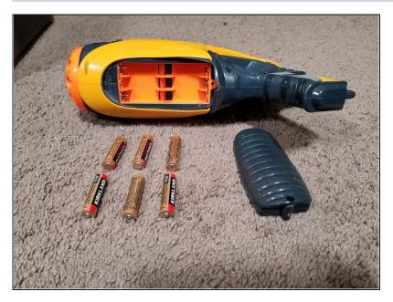
Remove the battery case using the Phillips head screwdriver and take out the batteries. You want to do this just in case something in the electronics goes haywire.
