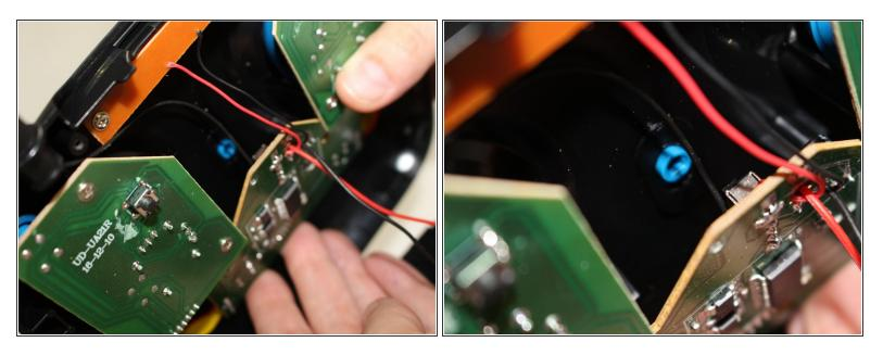
Move the motherboard up to allow room for the power bottom to become visible and loose.
