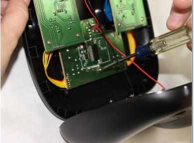
Remove the three 0.7mm Phillips #0 screws from the motherboard.
