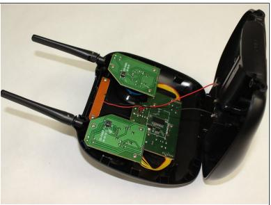
Remove the four 0.8mm Phillips #0 screws from the back casing of the remote.
