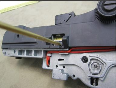
Now begin to remove the 3 2mm screws found on either side of the receiver.
