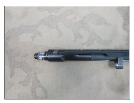
With the Barrel section removed the hop-up and the inner barrel can slide right out
