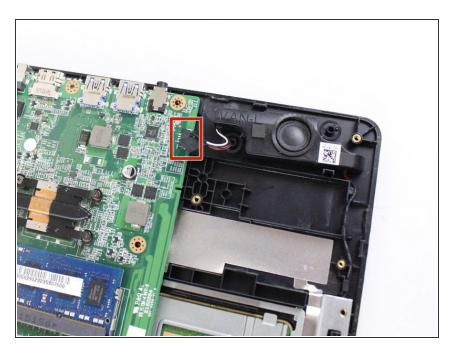
Remove speaker connector from the motherboard by pulling on the tab.
