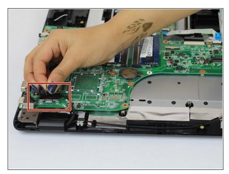
Remove screen connector by pulling it upwards.
