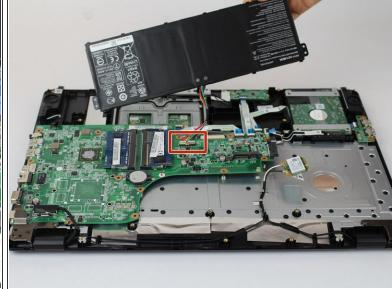
Remove the connector from the motherboard.
