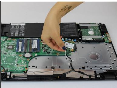
Remove wi-fi card by pulling from socket.
