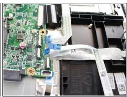
Remove the four blue tabbed ribbon connectors to the motherboard by lifting white clamps and pulling out connector.
