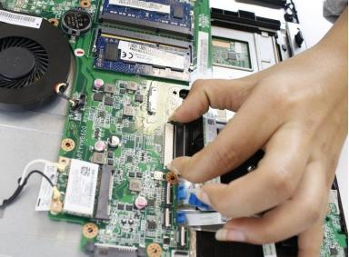
Remove black ribbon connector by lifting white clamp and pulling connector out.
