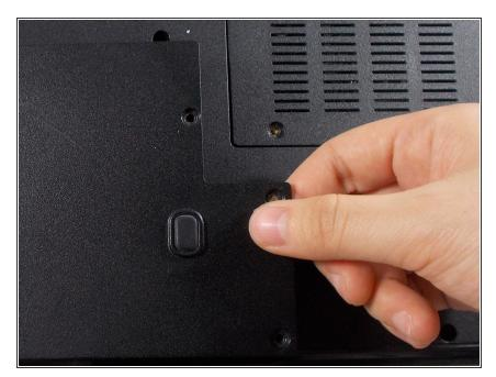
Lift back cover from the groove on the right side of the cover next to the symbol.
