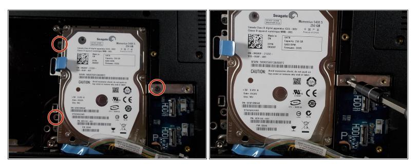
Remove the three Philips #1 3mm screws.
