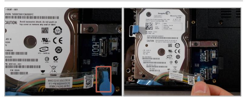
Pull up on the blue tab that is attached to the ribbon cable to unplug it.
