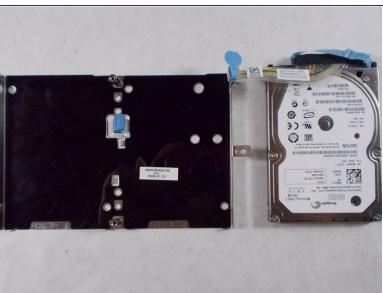
Remove the two 3mm screws with a Philips #1 screwdriver from the back side of the frame to remove the Hard drive.
