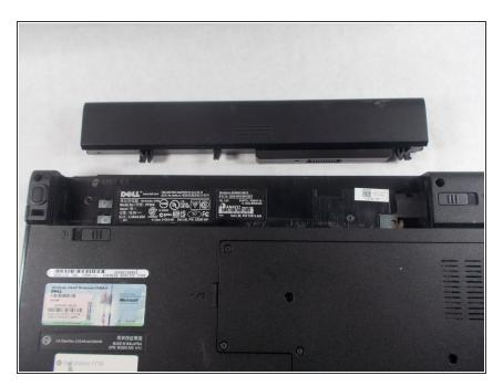
Remove the battery from the slot.
