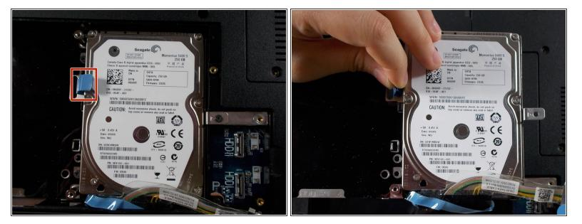
Lift and remove the Hard Drive frame by pulling up on the blue tab.
