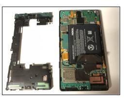
• Use the flat end of a spudger to pry the battery cover from the phone's frame.
