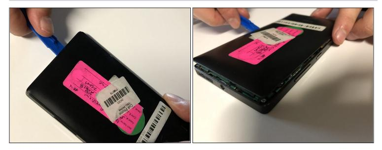
• Wedge a plastic opening tool between the two panels. Slide it along each side of the phone to completely remove the back panel.
