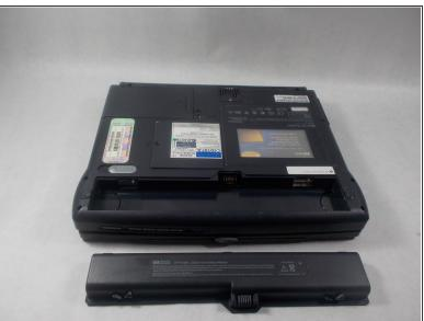
While continuing to hold the finger latch, slowly lift up on the tab to remove the battery from the device.
