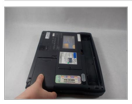
Once the button is unlocked to the side, slide the hard drive enclosure away from the device.
