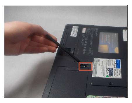
To unlock the hard drive, use a spudger to slide the button aside.
