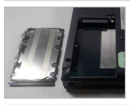
The hard drive will be clipped into the underside of the hard drive enclosure and can be removed for replacement.
