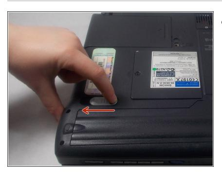
Slide the finger latch to the left to release the clip holding the battery into the laptop.
