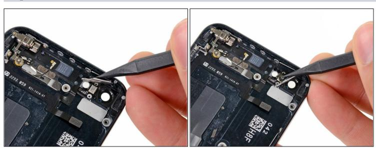
• Use the tip of a spudger to flip the metal bracket holding the power switch away from the top of the rear case.
