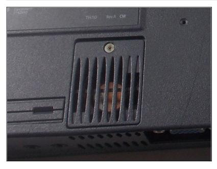
• Locate the fan on the underside of the laptop.
