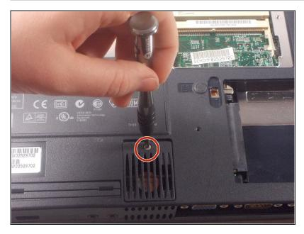
Using a Phillips #1 screwdriver, remove the 4.5 mm screw securing the fan cover to the device.
