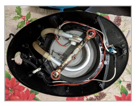
Taking out the 2 screws shown in the image unlocks the water heater, temperature regulator, and pot heater.
