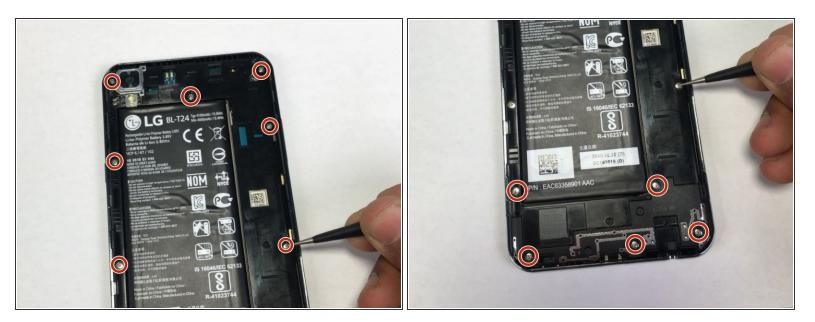
Remove the twelve 2.5mm Phillips #0 screws from the back of the phone.
