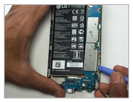
Insert a plastic opening tool underneath the motherboard and pry upwards to remove it.
