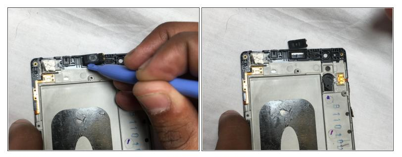
Using the plastic opening tool, pry off the ear speaker.
