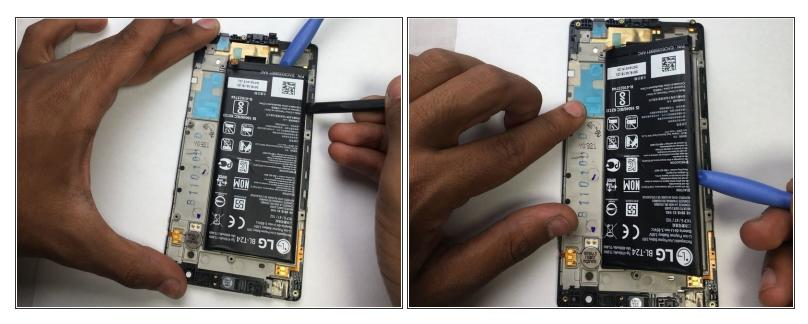
• Use a spudger and plastic opening tool to carefully pry up the battery.
