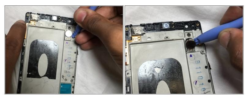
• Carefully peal off the glued vibration motor by using the plastic opening tool.
