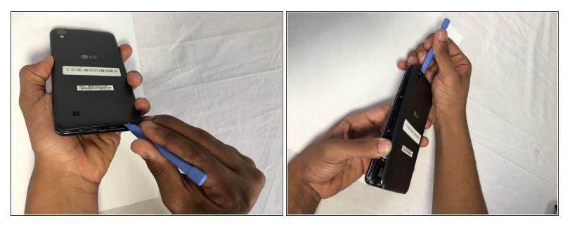
Insert a plastic opening tool above the AUX jack and slide it around the perimeter to pop the back cover off.
