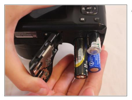
• Remove the batteries.
