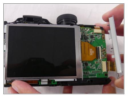
• Pull the small metal switch plate to the side.
