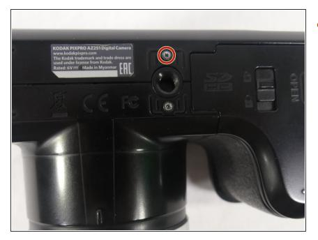
Remove the single 5mm Phillips #00 screw from the bottom.
