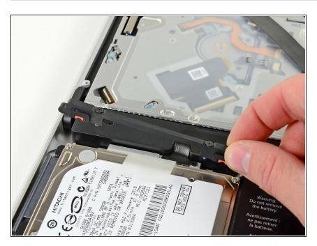
Lift the retaining bracket out of the upper case.
