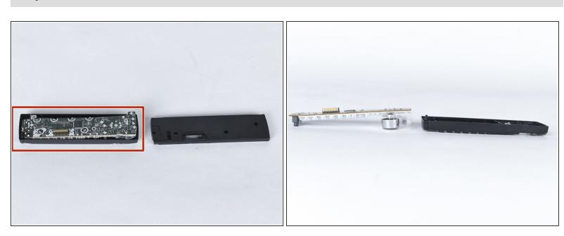
Remove the motherboard from the casing.
