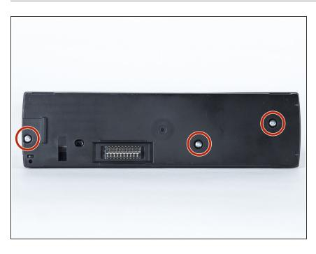
Use a Phillips #1 screwdriver to unscrew the three 3mm Phillipshead screws on the rear of the faceplate.
