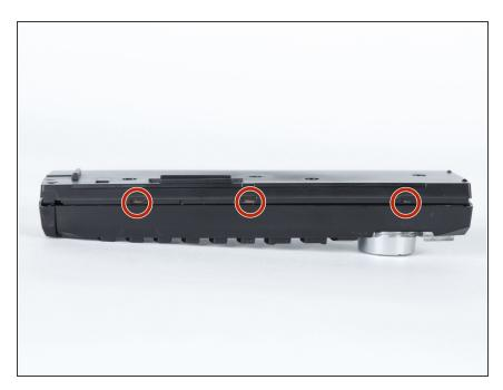
Press clips inward with the plastic opening tool to release the rear of the head unit.
