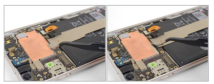
Use tweezers to peel up the tape at the top of the interconnect cable.
