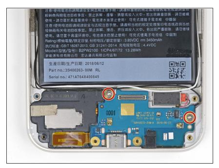
Remove the two 3 mm T5 screws securing the daughterboard to the frame.
