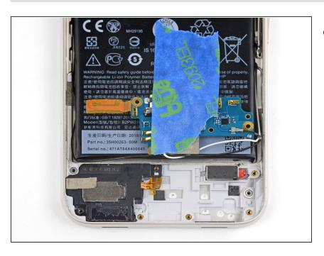
Flip the daughterboard over onto the battery and secure it out of the way with some tape.
