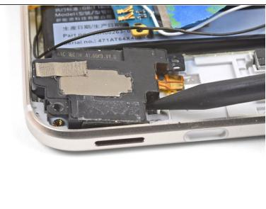
Use the point of a spudger to pry up and loosen the loudspeaker from its recess.
