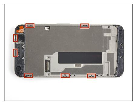
The midframe is held tightly in place by plastic clips which push into the edge of the back case.
