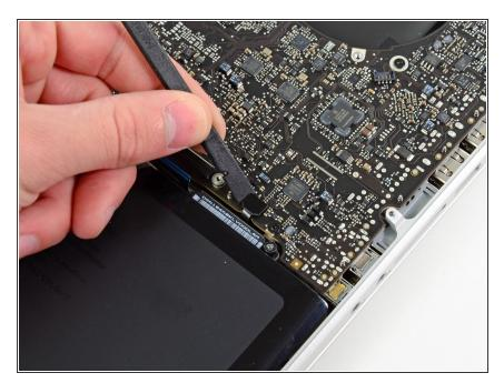
Use the flat end of a spudger to lift the battery indicator connector up and out of its socket on the logic board.
