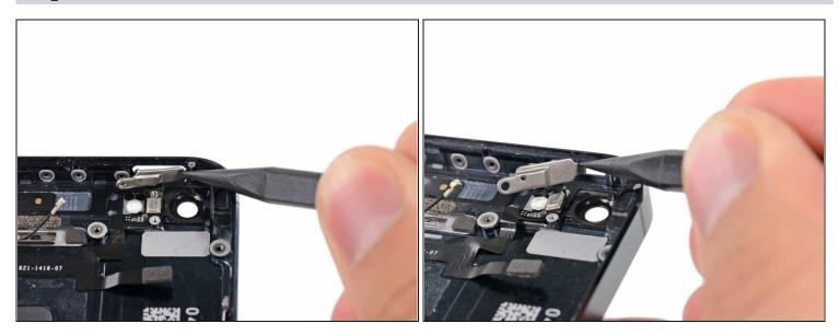
• Use the tip of a spudger to slide the power button bracket up and to the left to unhook it from the metal hinge.
