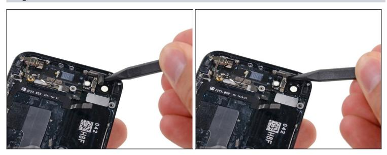
• Use the tip of a spudger to remove the rubber bumper from below the power button.
