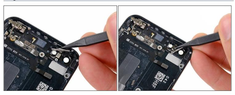
• Use the tip of a spudger to flip the metal bracket holding the power switch away from the top of the rear case.
