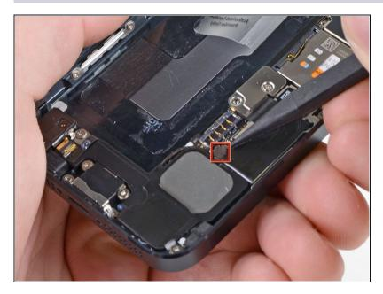
• Use the tip of a spudger to pry the cellular data antenna cable connector up from its socket on the logic board, just above the speaker enclosure.
