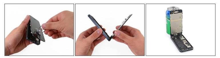
⚠️ Do not try to completely remove the front panel assembly from the rear case, as there are several ribbon cables still attached at the top of the iPhone.
