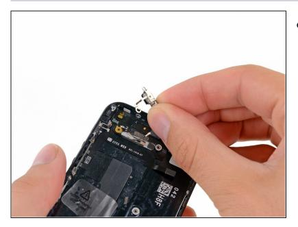
• Remove the vibrator and vibrator bracket from the rear case.
