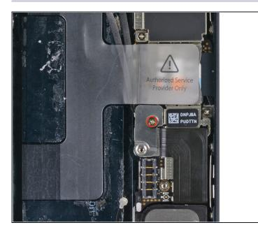
• Remove the single 1.2 mm Phillips screw remaining in the mid-section logic board bracket.
