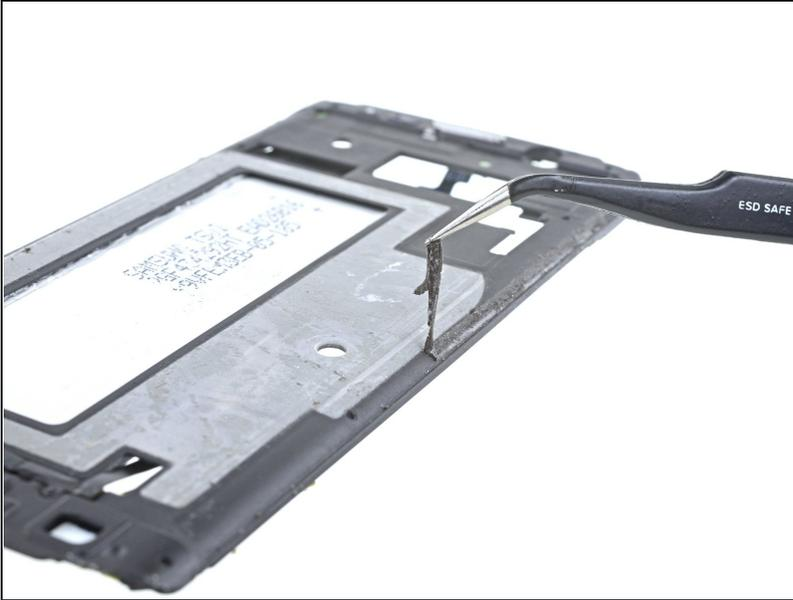
⚠ Before installing a new display, it's very important to remove all traces of the old adhesive from the frame, while taking special care to remove any small glass fragments.
