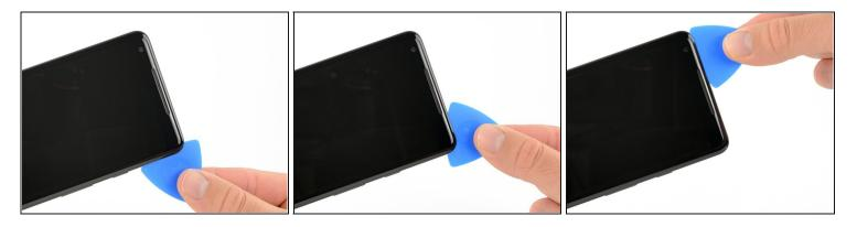
• Reinsert the flat edge of the pick at the top-right corner of the phone, and slide it around the corner and the top edge of the phone.
