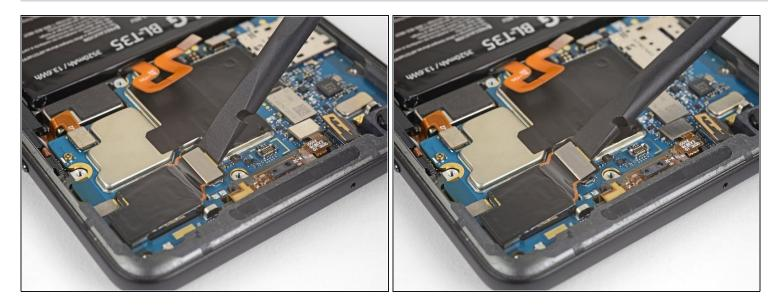
• Use the flat edge of a spudger to disconnect the rear camera connector.
