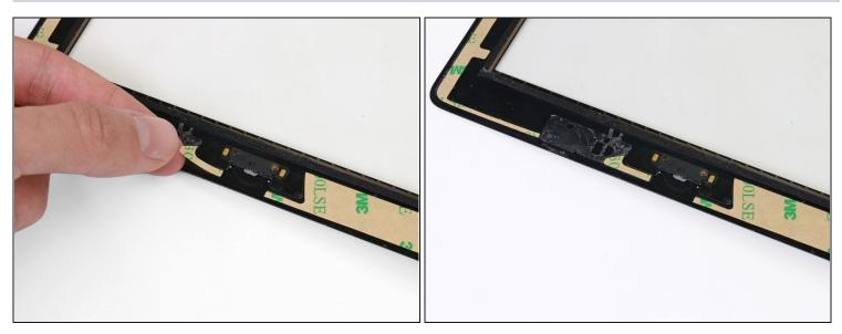
• Place the small hook-shaped adhesive strip below the left side of the home button mounting bracket.
