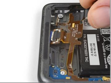
• Gently pull the USB-C port out of its recess in the phone case.
