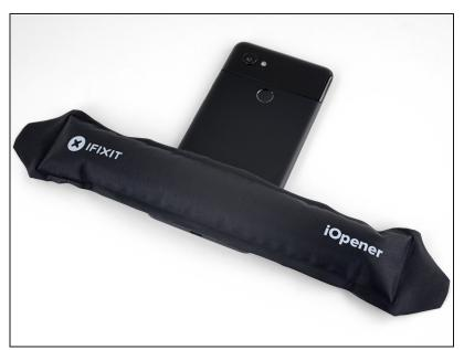
Use a hairdryer or heat gun, or prepare an iOpener and apply it to the bottom of the back of the phone for about a minute, in order to soften the adhesive securing the charging assembly.
