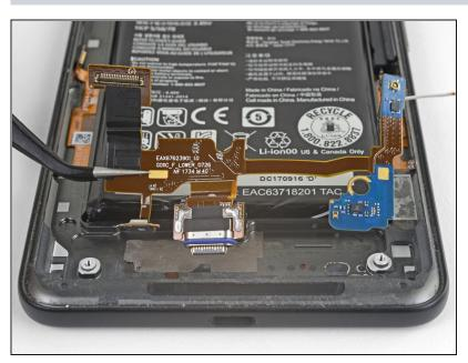
Lift the charging assembly out of the phone case. Compare your new replacement part to the original part—you may need to transfer remaining components or remove adhesive backings from the new part before installing.
