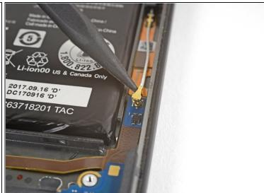
Use the point of a spudger to disconnect the white antenna cable to the right of the battery.
