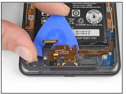
Starting from the left side, slide an opening pick under the charging assembly flex cable to separate it from the phone case.
