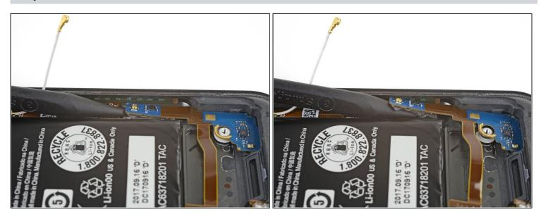
Slowly slide the point of a spudger underneath the antenna board to separate the adhesive tape under the board.
