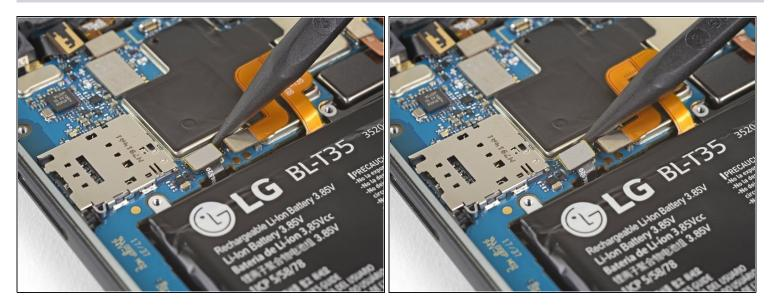
Use the point of a spudger to disconnect the fingerprint sensor connector.
