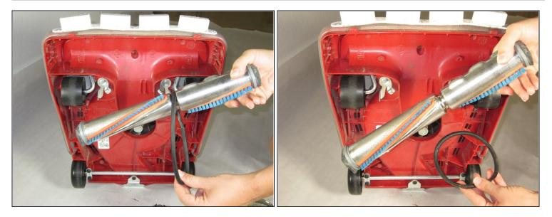
• Pull brush roller out and slip the belt off from the indent in the middle of the roller.
