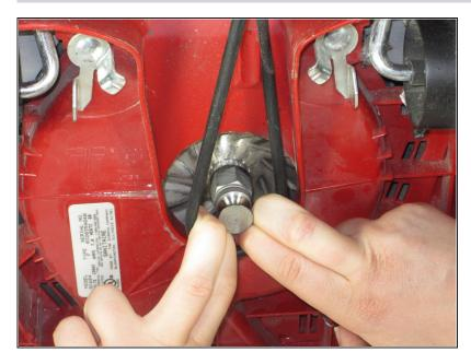
• Remove the belt from the circular knob by inserting your fingers on either side, gently lifting towards you.
