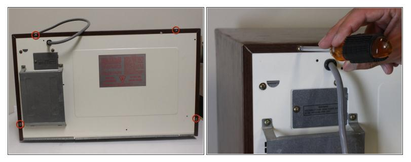
• Remove the additional four screws securing the wood-paneled case to the microwave frame.
