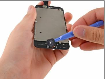
• Use a plastic opening tool to pry the home button up from the display assembly.
