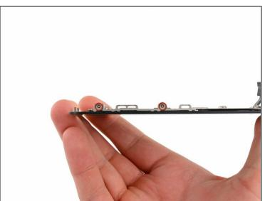
• Remove two 1.2 mm Phillips screws from each side of the LCD frame (four total).
