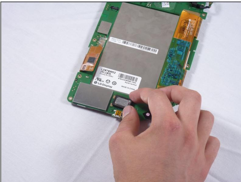
**⚠ When replacing the motherboard make sure that the speaker assembly component (small rectangular piece) is in place. It is not attached and needs to be properly aligned.**
