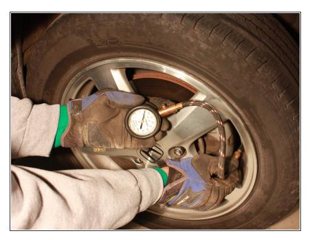
• Using an air compressor and the air pressure gauge, fill the front and rear tires to appropriate amount.
