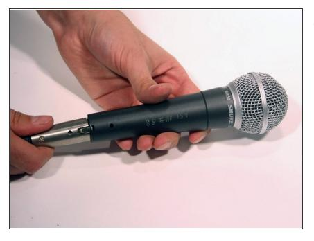
Once the pins are aligned, push the cable into the bottom end of the microphone. You should hear a click.
