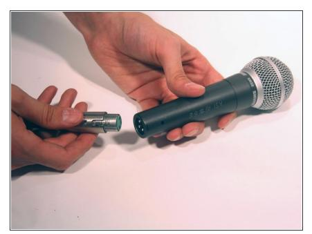
• Line up the pins in the end of the microphone (microphone connecter) with the holes in the XLR cable.
