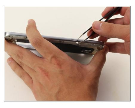
Push out the power button with the tip of the tweezers.
