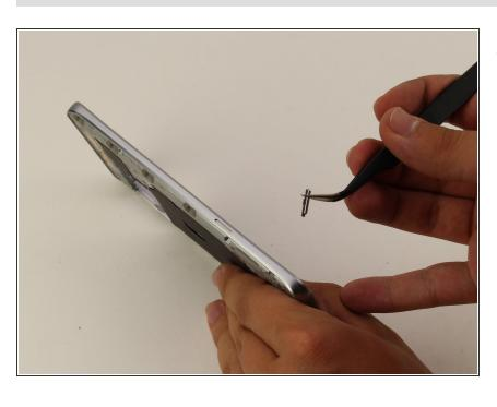
Push out the volume button and remove it from the device. To reassemble your device, follow these instructions in reverse order.
