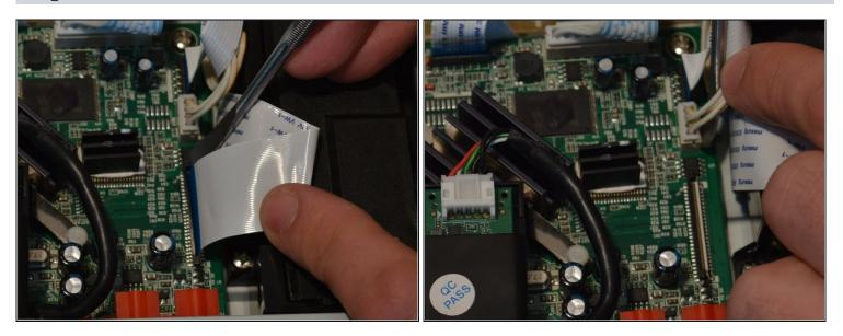
• Detach the tape wires from the motherboard and power board.
