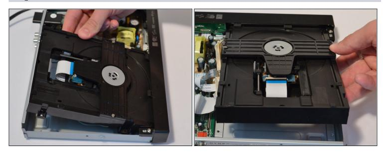
• Lift the disc drive up to a 45 degree angle and pull back out of the device shell
