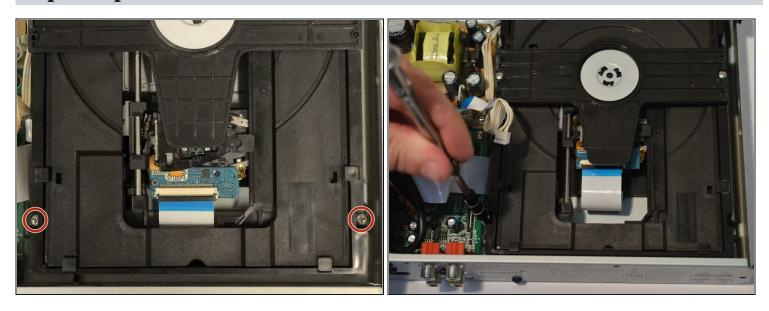
• Use a Phillips #1 screwdriver to remove the two screws that secure the Optical Drive.
