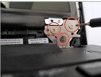
Loosen the marked screws.
