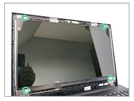
Remove the marked screws.
