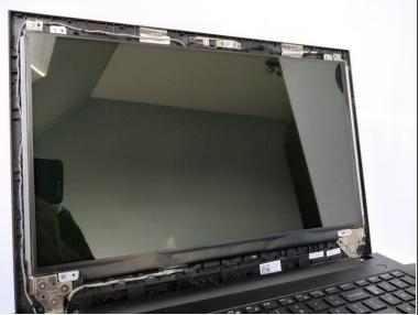
Use <u>Jimmy</u> or another opening tool to remove the screen bezel. Be careful not to damage the bezel.
