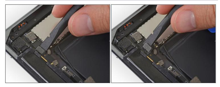
• Use the flat end of a spudger to lift the primary cellular antenna connector from its socket on the logic board.
