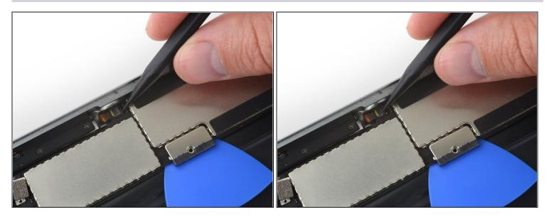
• Use the pointed tip of a spudger to flip up the retaining flap on the upper button assembly cable connector.
