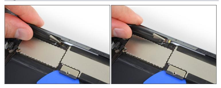
• Use <u>tweezers</u> to carefully pull the upper button assembly ribbon cable straight out of its connector.
