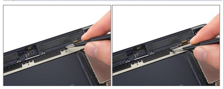
• Use <u>tweezers</u> to start peeling back the tape securing the upper component cable bracket.
