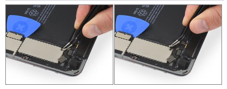
• Disconnect the antenna interconnect cable by lifting it straight up from its socket on the logic board.
