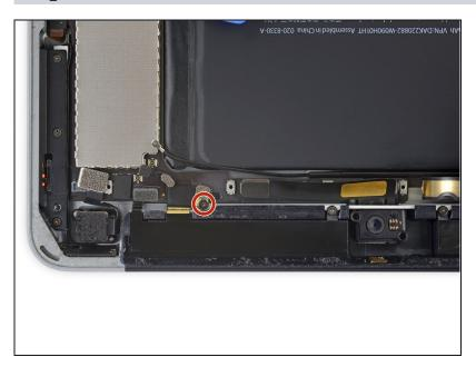
• Remove the 1.4 mm Phillips screw securing the primary cellular antenna interconnect cable bracket.
