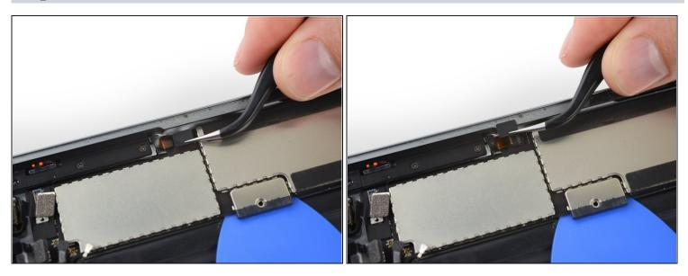
• Remove the piece of black tape covering the upper button assembly cable connector.
