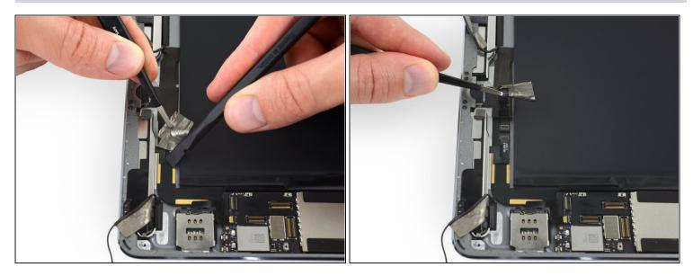
Peel the tape toward the home button to uncover the speaker cable connector.
