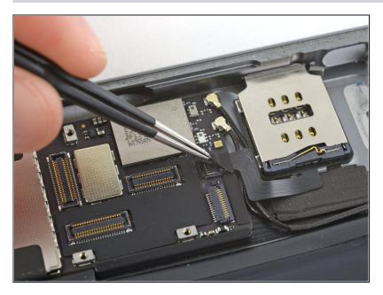
• Use <u>tweezers</u> to peel and remove the piece of tape covering the SIM board cable connector on the logic board.
