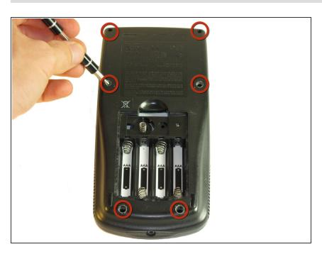
Unscrew the six 7.5mm T6 screws on the back case. You will need to use a screwdriver with a long and skinny head.
