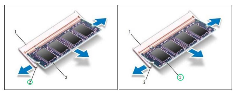
Use your fingertips to carefully spread apart the securing clips on each end of the memory-module connector until the memory module pops up.
