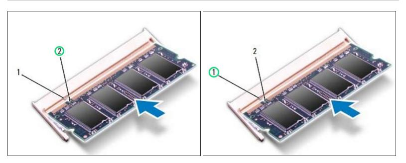
• Align the notch in the **NEW** memory module with the tab in the memory-module connector.
