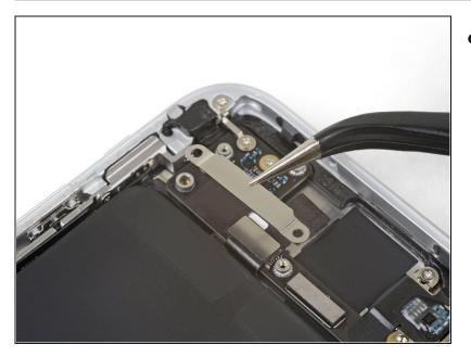
• Remove the upper cable connector bracket.
