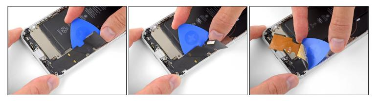
• Continue separating the Lightning connector assembly's flex cable until you pass the lower edge of the battery.
