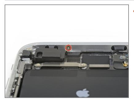
• Remove the 1.3 mm Phillips screw securing the antenna component to the top edge of the rear case.
