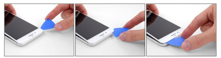
• Slide an opening pick underneath the display along the top edge of the phone to loosen the last of the adhesive.
