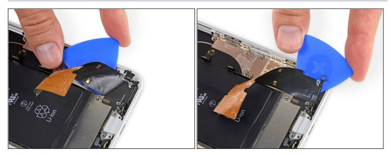
• Carefully slide your pick from the corner of the battery to the corner of the iPhone to separate the portion of the flex cable adhered to the outer frame.
