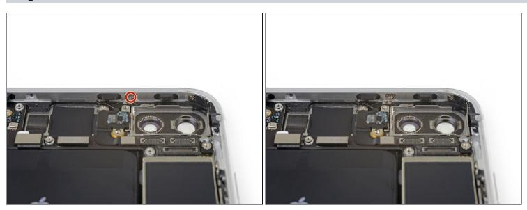
• Remove the 1.2 mm Phillips screw securing the antenna flex cable to the top edge of the iPhone's rear case.
