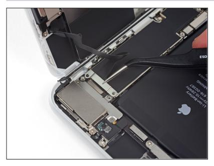
• Remove the bracket covering the front panel sensor assembly connector.
