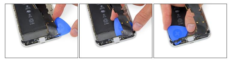
• Slide your pick across the width of the iPhone to separate all the remaining areas of the Lightning connector assembly from the rear case.
