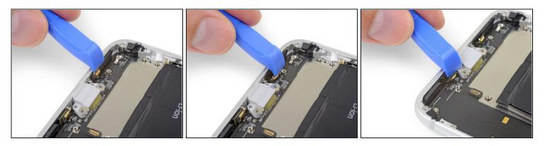
• Use the sharp edge of an iFixit Opening Tool to pry the two microphones free from the adhesive securing them to the lower edge of the iPhone.
