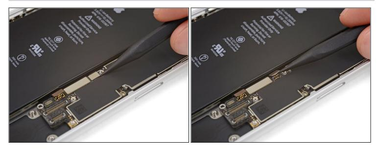
• Use the point of a spudger to carefully pry up and disconnect the wireless charging coil's flex cable.
