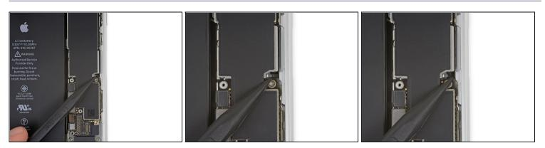
• Use the point of a spudger to push the SIM card eject plunger out of the logic board's way.
