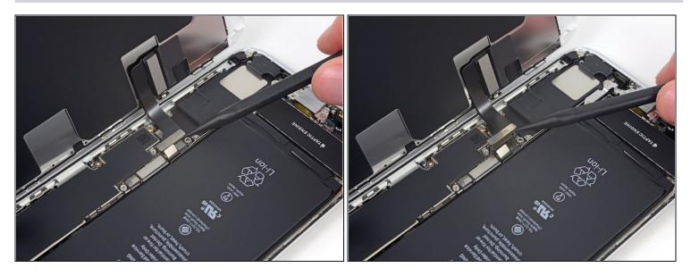
• Use the tip of a spudger or a fingernail to disconnect the large lower display connector by prying it straight up from its socket.
