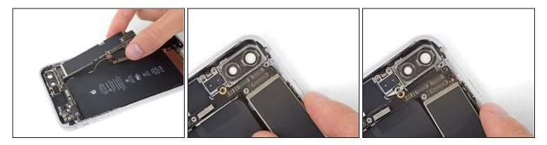
• Lift the logic board from the bottom edges and slide it toward the bottom of the iPhone to remove it.
