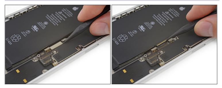
• Use the point of a spudger to pry up and disconnect the Lightning connector assembly's flex cable from the logic board.
