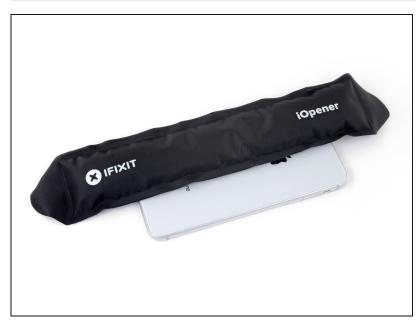
Apply an iOpener or use a hair dryer to heat the rear case behind the Lightning connector flex cable. This will soften the adhesive securing the flex cable, making it easier to separate.
