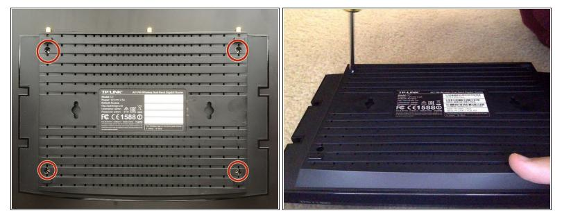
• Remove the 4 screws that secure the top cover of the router to the base.
