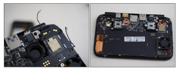
• Remove Wi-Fi antenna cable and LCD connector
