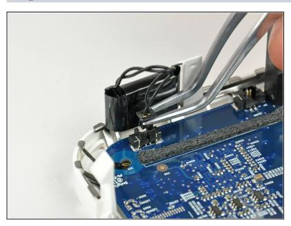
• Firmly grasp the sleep light cable connector with a pair of tweezers and lift it straight up off the logic board.
