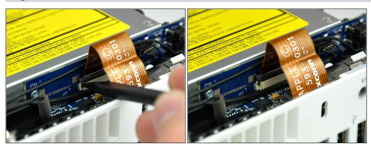
Use the tip of a spudger to slightly lift the left side of the ZIF cable lock up from its socket.
