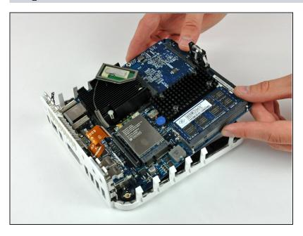
Gently lift the free end of the logic board and wiggle the board as you pull it away from the I/O ports.
