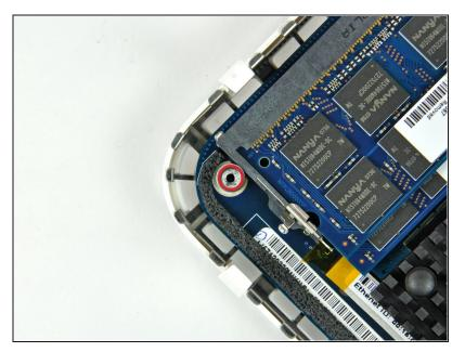
Remove the single T10 torx lug securing the logic board to the bottom housing.
