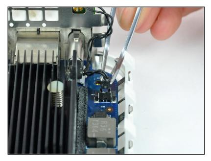
Firmly grasp the power button cable connector with a pair of tweezers and lift it straight up off the logic board.
