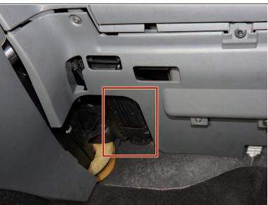
The cabin air filter is located in the passenger side footwell
