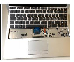
Insert a small screwdriver into the holes the screws were removed from in the previous step to unclip the keyboard.
