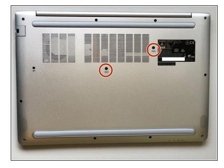
Remove the two keyboard retaining screws.
