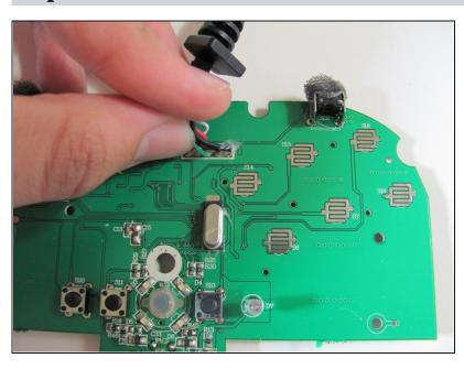
Locate the broken or disconnected wire by gently pulling up on the five wires connected to the motherboard
