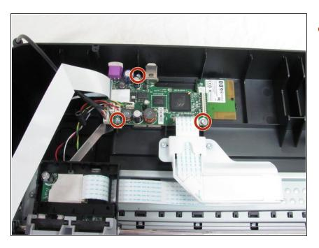
Remove the three uncovered T10 screws from the motherboard.
