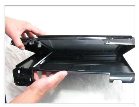
Pull the printer hood upward.
