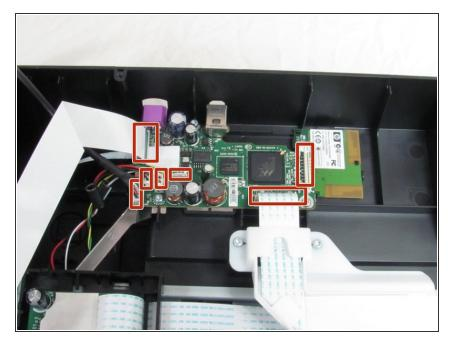
Gently remove the seven cables that are attached to the motherboard using a plastic opening tool.
