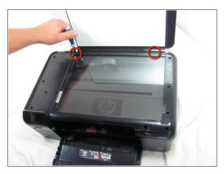
Use a T10 screwdriver to unscrew the two screws that fasten the frame to the printer hood.
