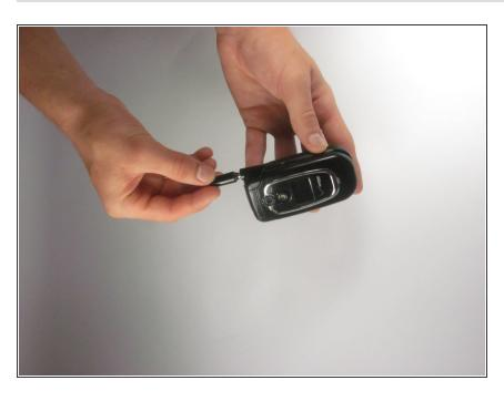
Twist the base in a counterclockwise motion to unscrew the antenna.
