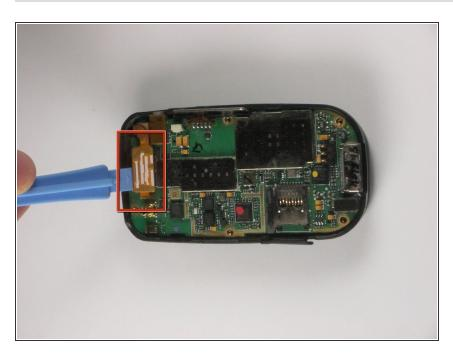
Detach the highlighted piece from the logic board using a plastic opening tool.
