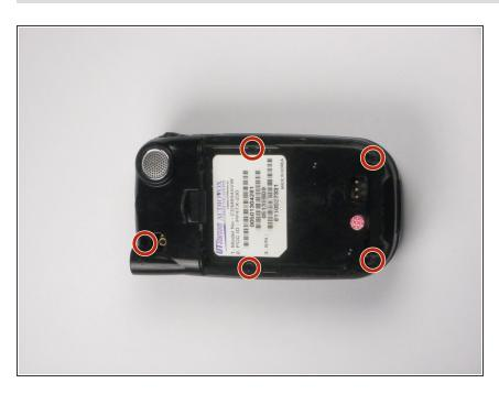
Remove five screws using a Phillips #00 screwdriver.
