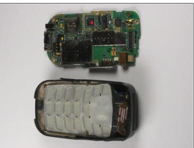
Remove the logic board from the anterior piece of the outer case using the plastic opening tool.
