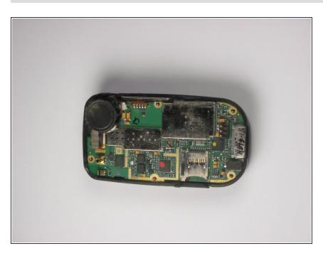
Remove the back piece of the outer case.
