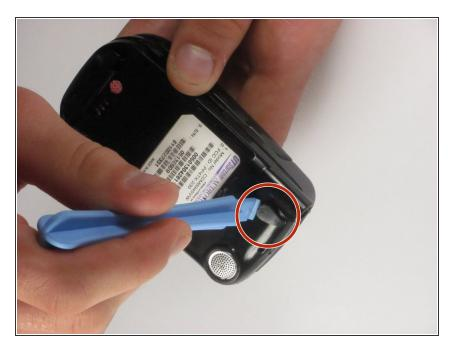
Remove the small rubber grommet using the plastic opening tool.
