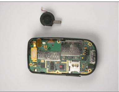
Remove the wire attached to the speaker from the motherboard using tweezers.
