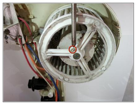
Remove the screw that is holding the fan to the motor using a Phillips screwdriver.
