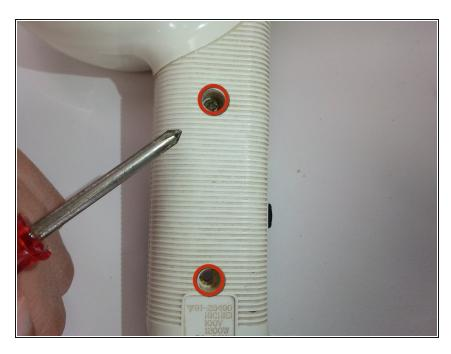
Locate the screws on the handle and remove with a Phillips screwdriver.
