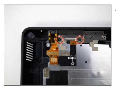
Remove the two 2.1mm T5 Torx screws from the volume button retaining bracket.
