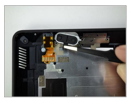
• Remove the volume button from the rear panel.
