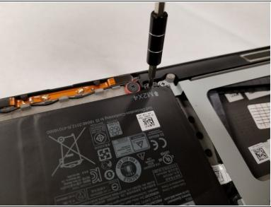
Remove the four 4.0 mm JIS #0 screws surrounding the battery.
