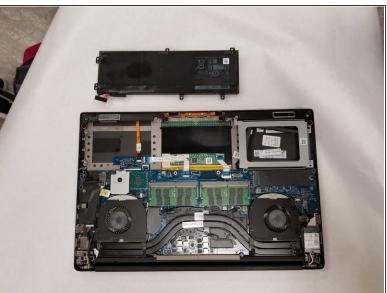
Carefully remove the battery from the computer.
