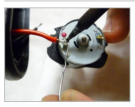
Using a soldering iron, solder the wires onto the new motor.
