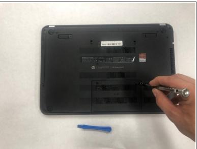
Remove the two #1 Phillips 4mm screws that hold the cover in place.
