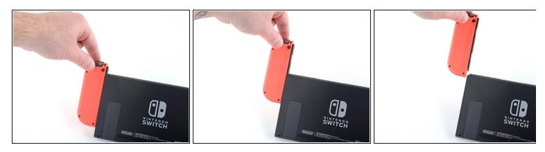
• Continue sliding the Joy Con upward until it's completely removed from the console.
