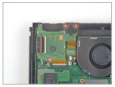
Use a JIS 000 screwdriver or an official iFixit PH 000 driver to remove the three 3.1 mm screws securing the headphone jack and game card reader board to the device.
