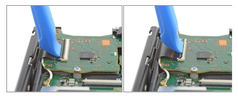
• Use an opening tool or your fingernail to flip up the small, hinged locking flap on the digitizer cable's <u>ZIF connector</u>.
