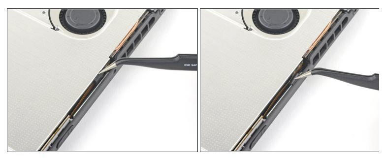
Use your fingers or a pair of tweezers to peel back the piece of foam on the top edge of the device near the fan exhaust port.
