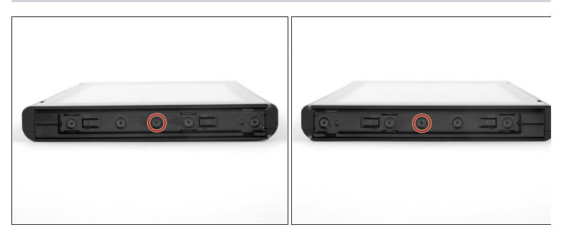
Use a JIS 000 screwdriver or an official iFixit PH 000 driver to remove the two 3.8 mm center screws on the sides of the device (one on each side).
