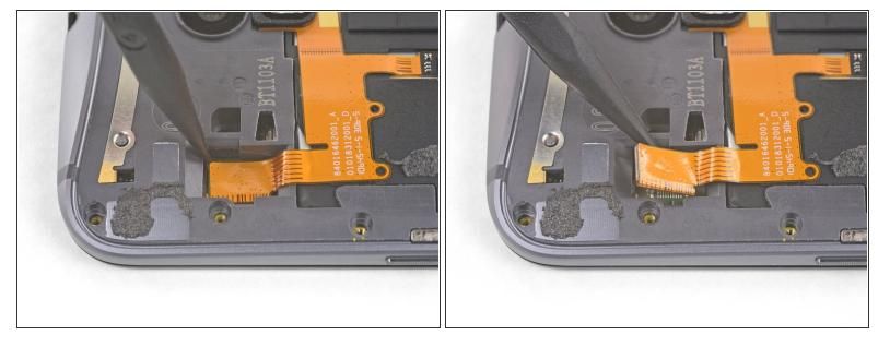
• Use the tip of a spudger against the corner of the flash connector to pry the connecter straight up and out of its socket.
