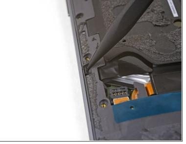
• Use the point of a spudger to push the small clip securing the left side of the midframe toward the edge of the phone, releasing the clip.
