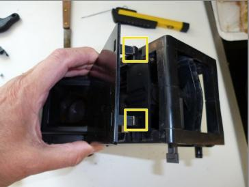
• Unclip the upper protection panel, then remove it by lifting it up.
